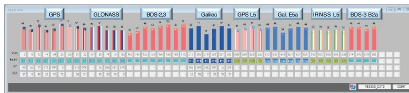
FIGURE 3 Screenshot of the L1-L5 TeseoAPP configuration, from the ST Teseo-Suite tool (using the Naples rooftop antenna).
