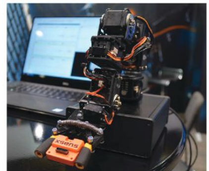
XSENS' AUVSI BOOTH: A robotic arm manipulates the MTi 600 while a laptop displays position information.
